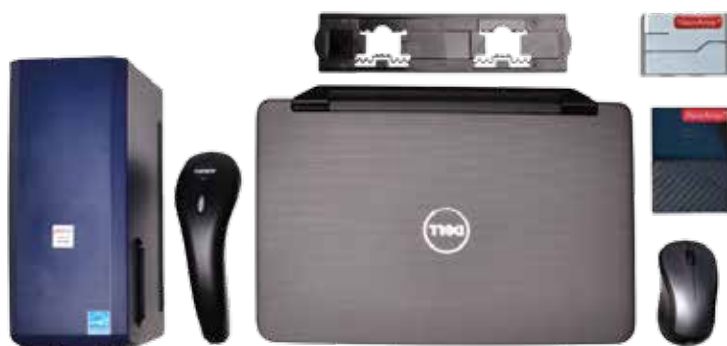
Scanner 8100; Slide Holder SingleScan; Hand Scanner; PC with preinstalled VisionArray Analyzer Software SingleScan; USB-Hub; External Hard Drive; Computer Mouse
